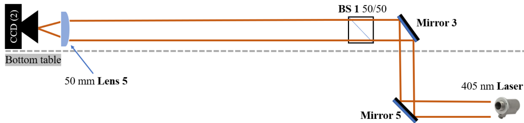
Figure 10 - Schematic of the procedure to align Lens 5.
