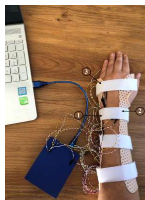
Figure 8: Experimental setup and implementation of the whole prototype. Pressure and temperature values were obtained at the end of ulna (1), at the distal end of radius and near the anatomic snuffbox (2) and at the most prominent point of the abductor digiti minimi (3).
