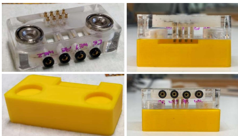
Figure 3.7 Switch box fabricated at CENIMAT I3N to interface the dual detection LIG devices with the potentiostat.
