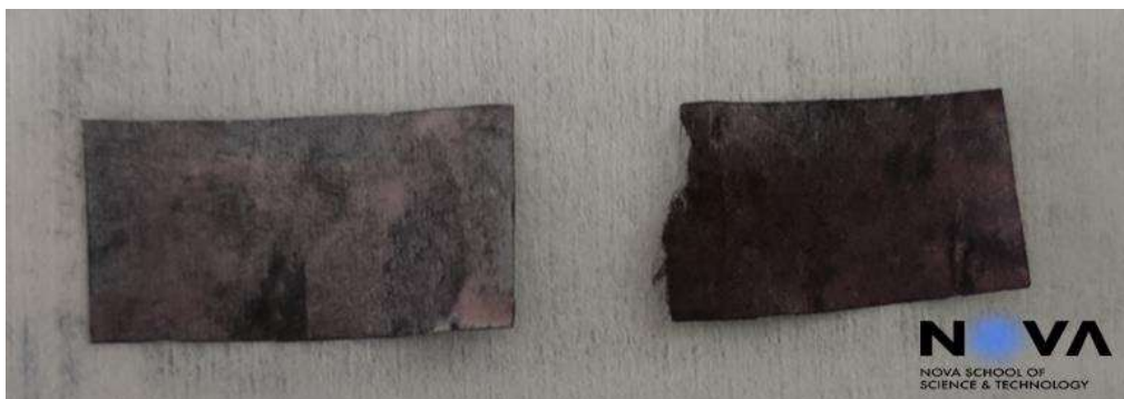
Figure 4.22 Pictures of resulting membranes produced with the optimized method: right (office paper) and left (cardboard substrate).
