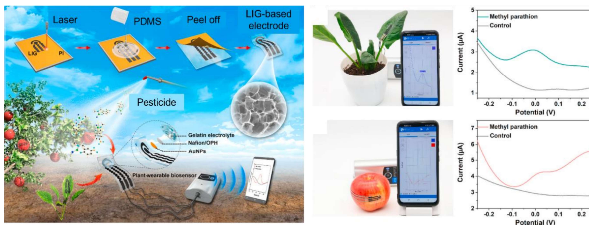
Figure 2.27 Schematic representation of the fabrication process of LIG onto PI and transference to PDMS, and respective functionalization, and photographs and electrochemical results of in-situ analysis of methyl parathion on the surface of different agricultural products (spinach and apple). Adapted from Zhao, F., 2020. 255
