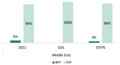
Figure 20 - Middle East BOF and EAF penetration rates in 2050 by scenario
