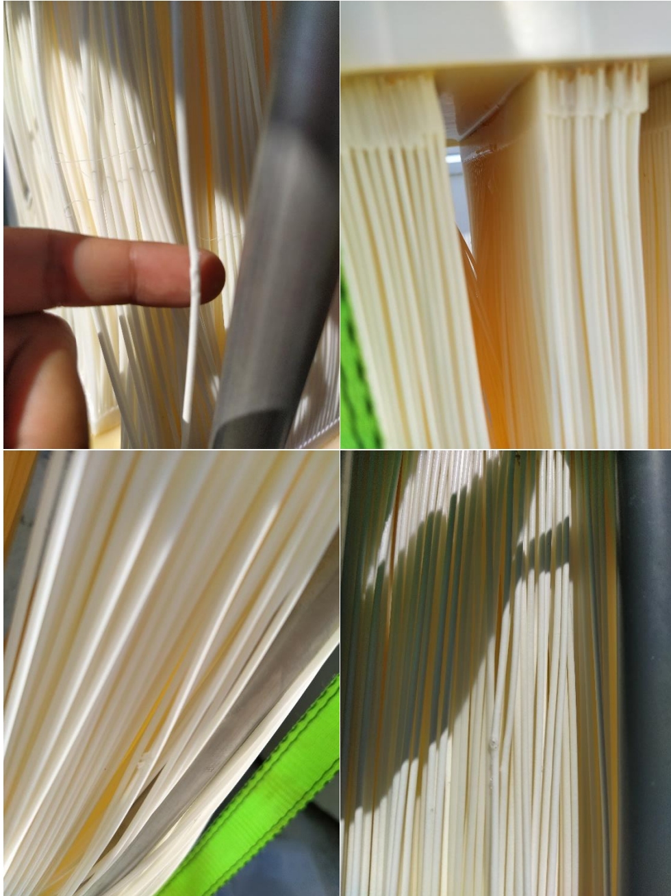
Figure 4.9 – Bundles torn up.
