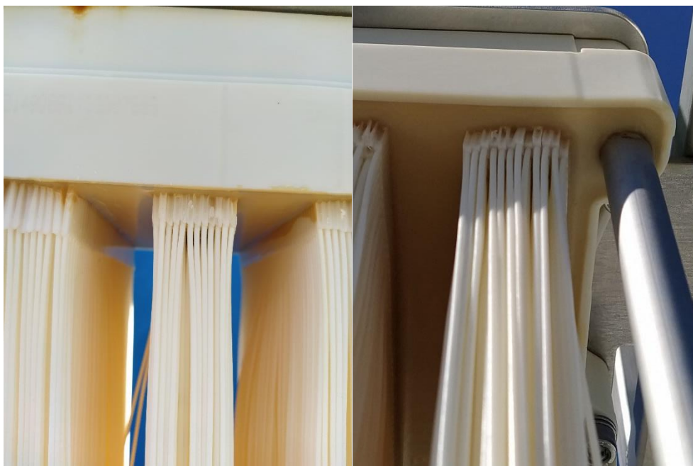
Figure 4.7 – Top and bottom of the membrane that is glued to the support.
