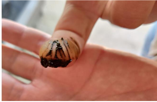
Figure 4.2 – Dirt that came out of the membrane after several days of cleaning.
