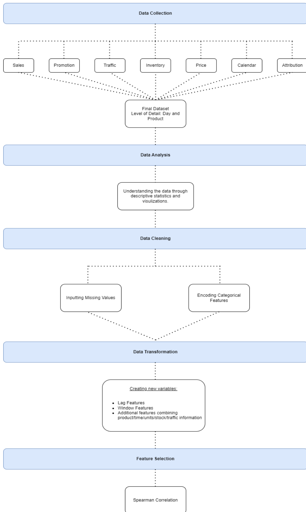
Figure 5 - Workflow of the Data Collection, Analysis, Preparation, Cleaning, Transformation and Feature Selection
