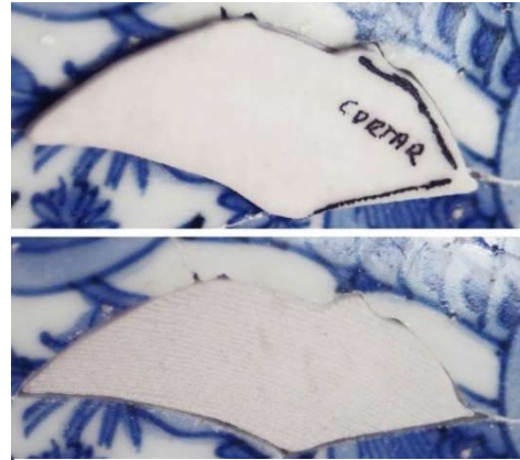
Figure 3.14 - Comparison between a 3D printed filling before and after sanding.
