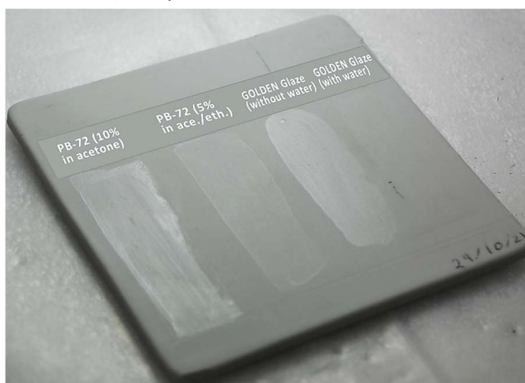
Figure 3.34 - Testing of different materials for creating a barrier layer.
