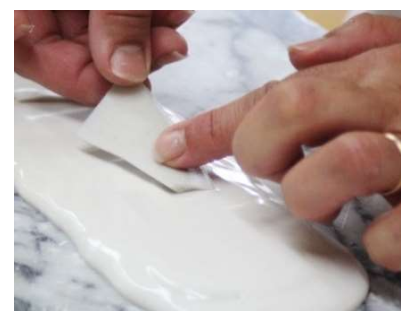
Figure 3.17 - Pressing a filling on poured plaster to create an underlaying support.
