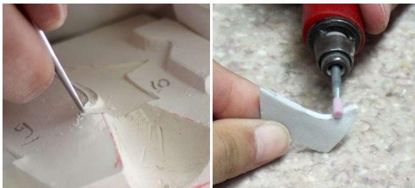
Figure 3.26 - Adjustment of a fragment’s mould (left) and grinding of the fired fragment (right).
