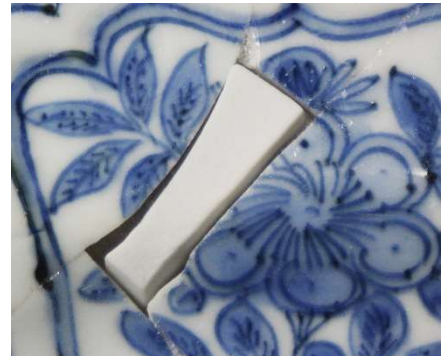
Figure 3.25 - Detail of a porcelain filling in need of extra material.
