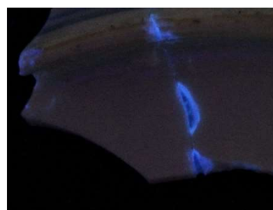
Figure G.1 - Detail of the adhesive-residues fluorescing under U.V light.
