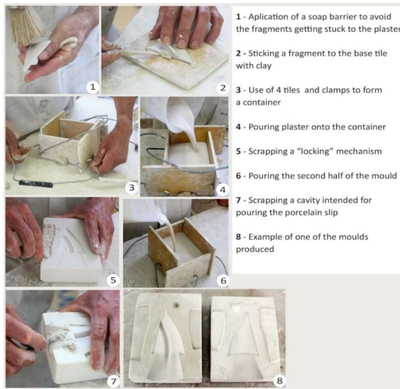
Figure 3.15 - Mould-making process.
