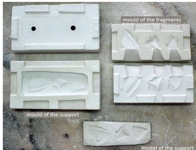
Figure 3.18 - Example of a mould of a group of fillings (right), and the respective mould (left) of their support model (below).
