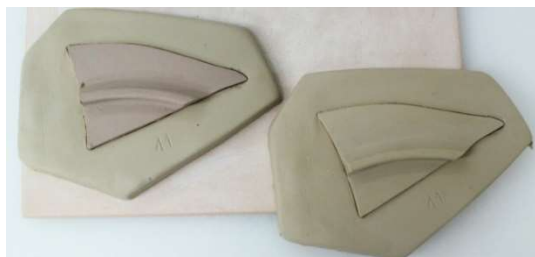
Figure 3.21 - Example of two fillings casted in "Chinese slip" (left) and white slip (right), both placed in their respective casted supports.
