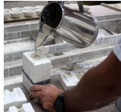
Figure 3.19 – Slip casting of a filling.
