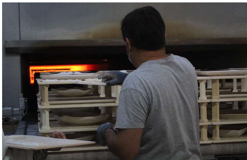
Figure 3.24 - Placement of the fillings in the oven.
