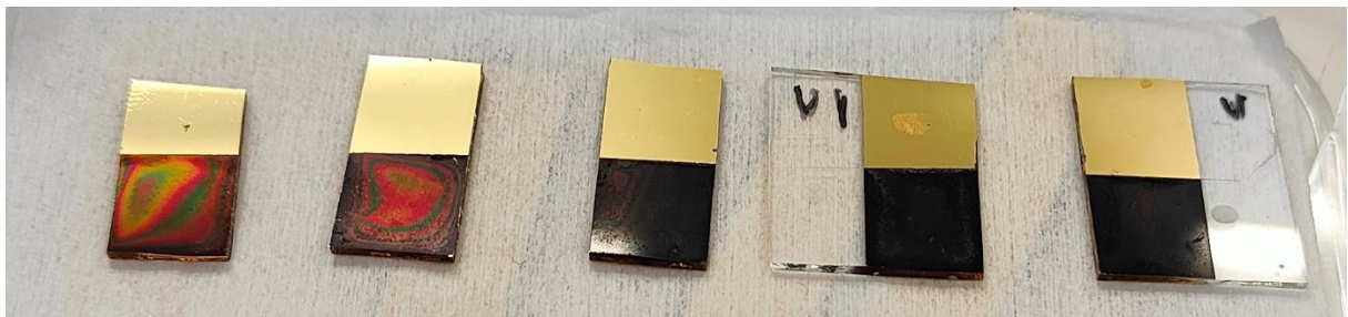
Figure 3.6- Electrodeposited MnO 2 samples obtained at deposition intervals of 60 s, ranging from 1 to 5 min (left to right).
