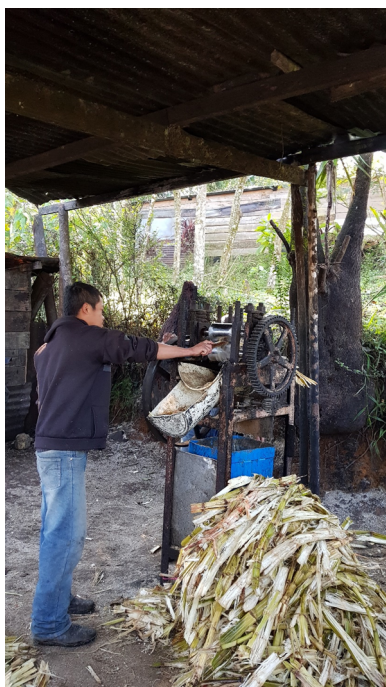
Figure S1. Sugarcane juice extraction during the artisanal production of Boj in Cobán, Guatemala.
