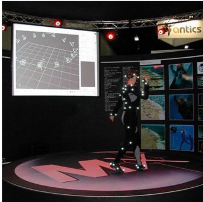
Figure 2.20 - Motion capture using visible light and an array of 16 cameras
