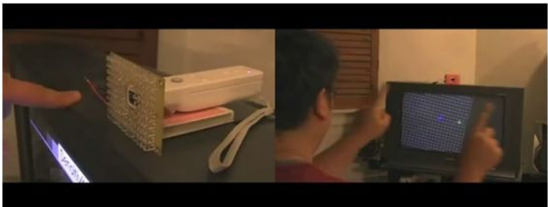
Figure 2.3 - Tracking fingers with a Wiimote
