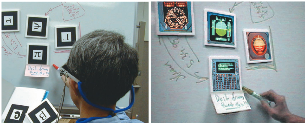
Figure 2.9: Collaborative tangible interface, combining virtual elements with real world annotations. Non-augmented view of collaborative AR interface (left), augmented view of collaborative AR interface (right) [41].
