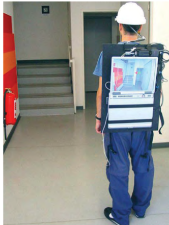
Figure 2.3: Notebook being used as a backpack computing platform displaying debug info, coupled with HMD [11].
