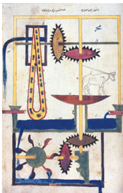
Figura 57. Al-Jazari's hydropowered saqiya chain pump device. The art & science of water, 2016.
