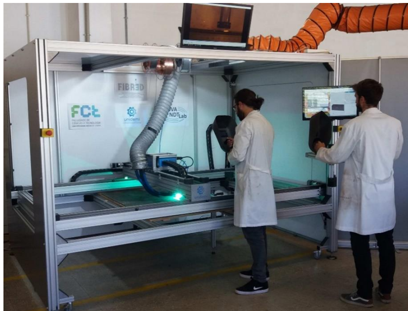
Figure 3.3 - Photograph of the developed 3 axis 3D printer
