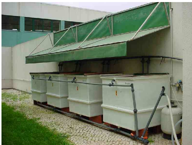
Figure IV.1: Experimental tanks at the sewage treatment plant.
