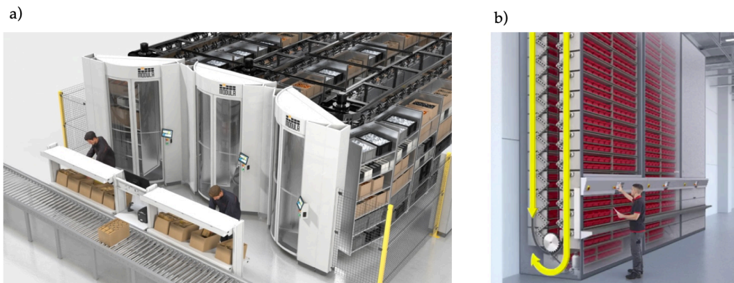
Figura 3.14 – a) Carrossel horizontal b) Carrossel vertical [40, 41]
