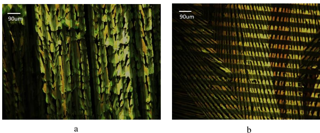
Figure 3.8: Microscope pictures of a) TIPS based detector and b) TIPGe based detector on glass.
