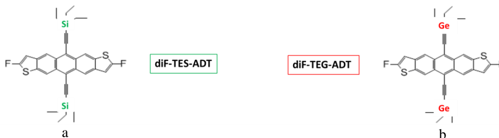
Figure 1.6: a) diF TES ADT molecular structure and b) diF TEG ADT molecular structure.
