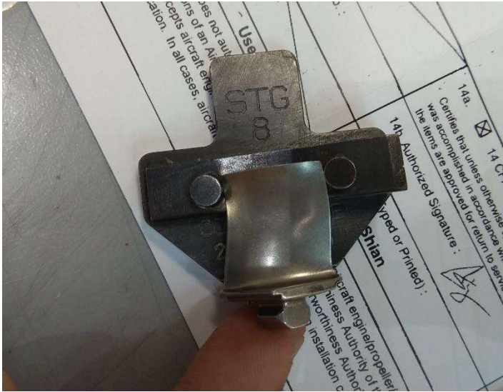
Figure 2.10 - Go/No Go Tool for Chord Length Dimensional Inspection
