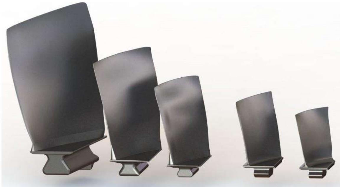
Figure 7.3 - Rendered Image of HPC Blade's CAD Reference Models (Stages 1 to 5)
