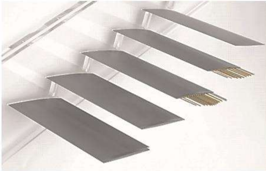
Figure 3.5 - Airfoil Cascade Arrangement Experiment [8]
