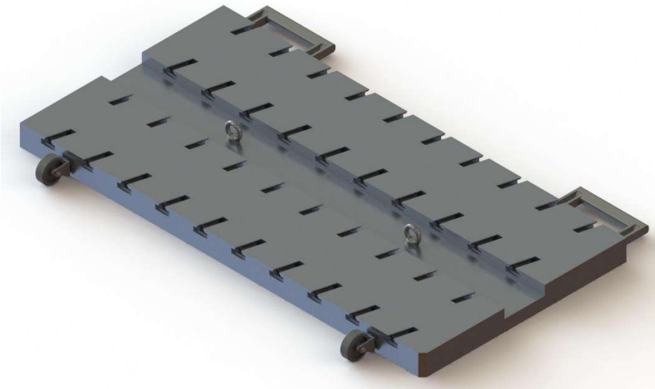
Figure 5.63 - 1 st Stage Tool with Handle Bars and Caster Wheels
