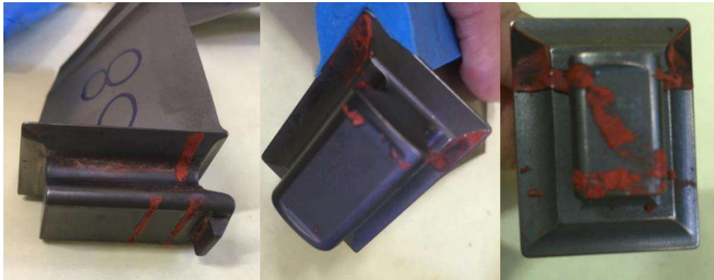
Figure 5.4 - HPC Blades with damaged RTV Silicone
