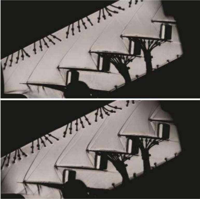
Figure 3.7 - Schlieren Photograph from Cascade Experiment [8]
