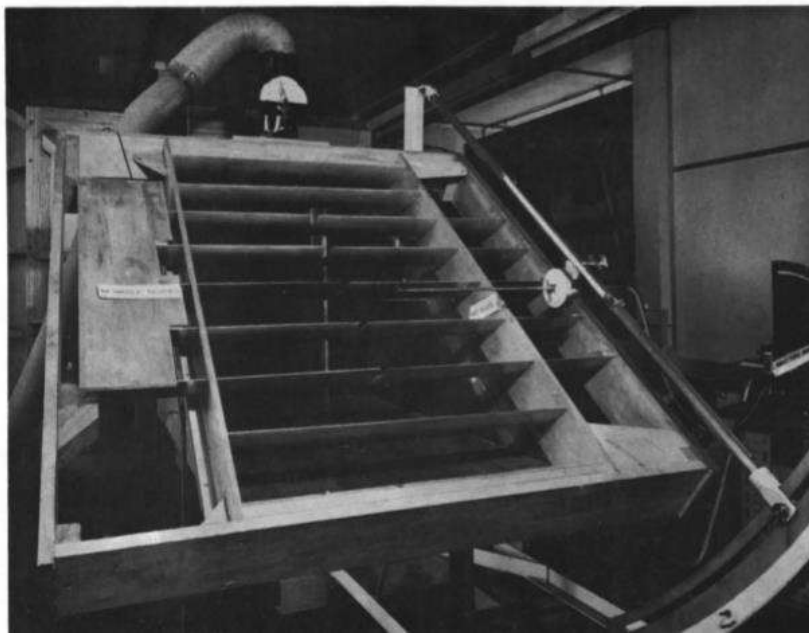
Figure 3.9 - Cascade Arrangement Experiment to study secondary flows [10]
