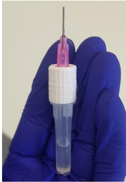
Figure 5.8: Collection kit 2 (STAB VIDA) for the collection and incubation of feather tips in 500 \mu\text{L} of Sample collection Buffer A.
