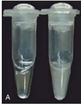
Figure 1.4: Endpoint detection of LAMP products by turbidity analysis. The tube on the left represents a negative result, and the tube on the right a positive. Adapted from Mori et al (2009) 27 .
