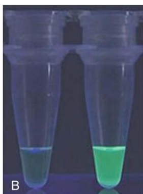
Figure 1.6: Endpoint detection of LAMP products using intercalating dyes such as calcein, under the UV/light. The tube on the left represents a negative result and the tube on the right a positive. Adapted from Mori et al (2009) 27 .
