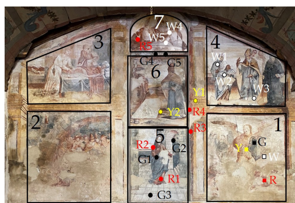
Figure 2. Location of the analysed colours with portable i-Raman (circles) and detached areas of sampling (squares) in Nossa Senhora das Neves Chapel mural paintings. G = grey, W = white, Y = yellow, and R = red.
