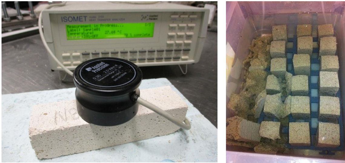
Figure 4. Prismatic samples being tested for thermal conductivity (left) and resistance to sulphates (right)
