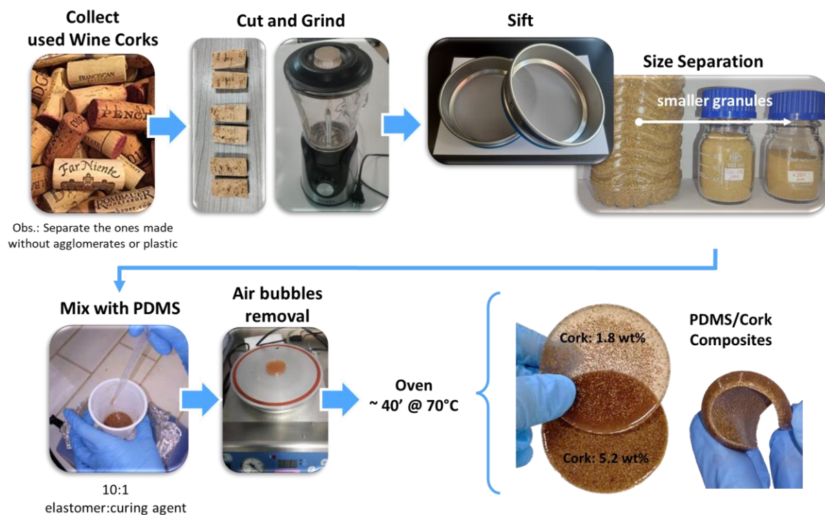
Figure 5.8 - Schematic of the production steps to obtain the PDMS/Cork composite samples, from the cork wastes grinding to the manipulation process of PDMS. Examples of final samples with cork granulates <500 \mu\text{m} , varying the wt% of cork.
