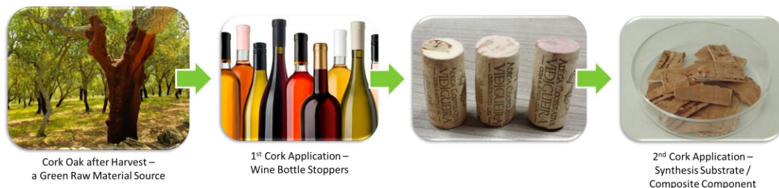
Figure 6.5 - Giving cork a second life: Use wine bottle stoppers wastes as a raw material for a new application.
