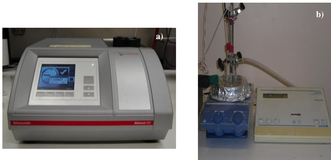
Figure 2.3. a) Anton Paar ABBEMAT 500 automated refractometer and b) Radiometer Analytical CDM210 conductimeter.
