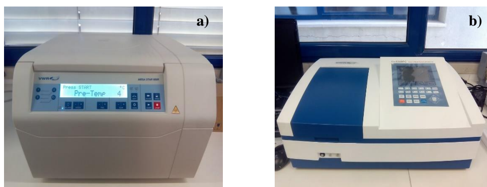
Figure 3.3. a) VWR® Mega Star 600 R Centrifuge and b) VWR® spectrophotometer, model UV-6300PC.
