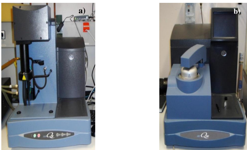
Figure 2.1. a) TA instrument Model TGA Q50 used for the measurements and b) TA Instrument Model DSC Q200 used for the measurements.
