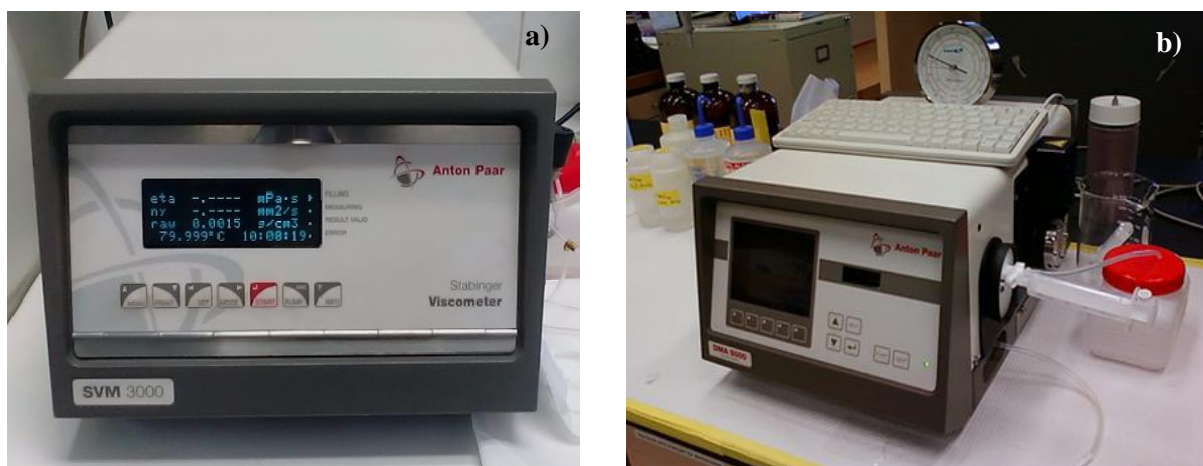
Figure 2.2. a) Anton Paar SVM 300 used for viscosity measurements and b) Anton Paar DMA 5000 densimeter used for density measurements.
