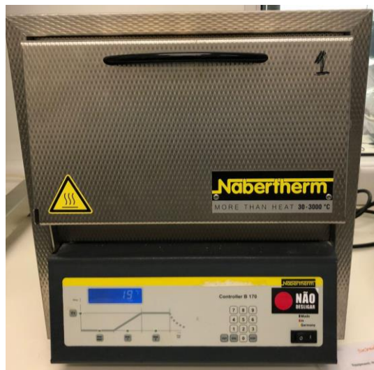
Figure 32- Picture of the Nabertherm furnace used to anneal NiO x .
