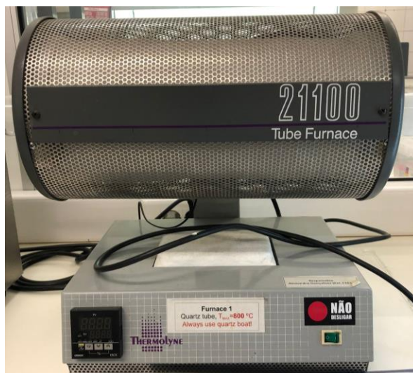
Figure 33- Picture of tube furnace used to anneal NiO x .
