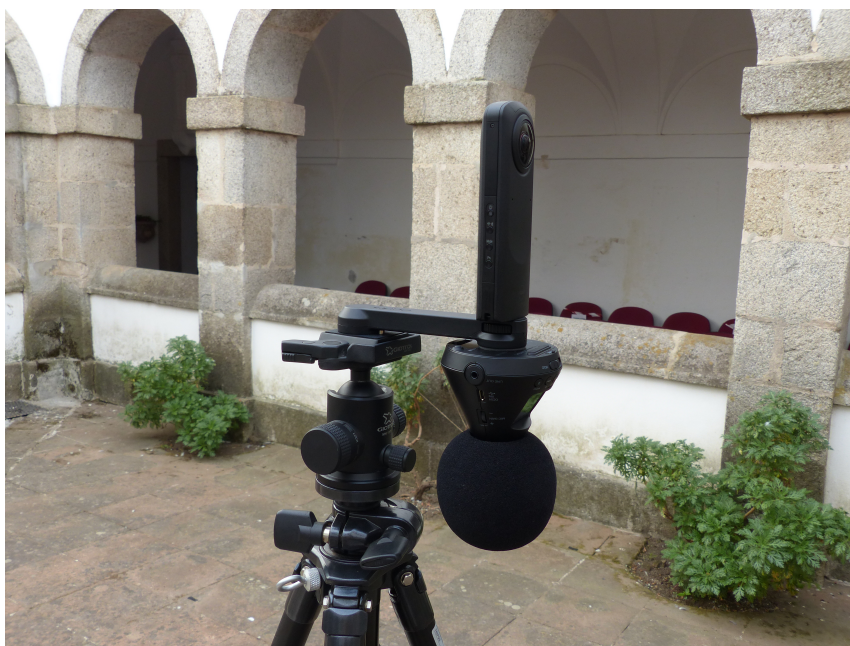
Figure 4.10: Recording setup consisting of a tripod with a camera on top and a microphone on the bottom, in Remédios Convent's cloister.
