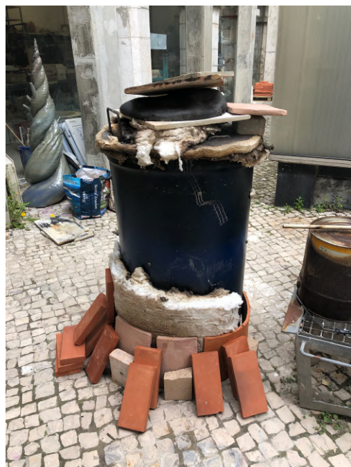
Appendix figure 5, After the wood is introduced the kiln is sealed off to keep out oxygen, Photo by the author.
