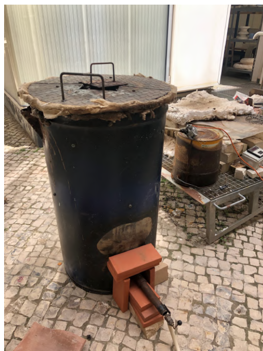
Appendix figure 2, The piece is inside the kiln, temperature is brought up to 600. Photo by the author.
