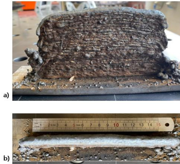
Figure 3.7 - Wall 1 (Deposited State): a) Front view; b) Top view
