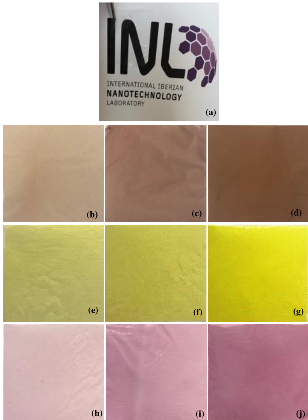
Figure C.1.3.1 – EC-based films with (a) 0% (w/w) natural dye, (b) 0.5% (w/w) anthocyanins, (c) 1% (w/w) anthocyanins, (d) 2% (w/w) anthocyanins, (e) 0.5% (w/w) curcumin, (f) 1% (w/w) curcumin, (g) 2% (w/w) curcumin, (h) 0.5% (w/w) betalains, (i) 1% (w/w) betalains, (j) 2% (w/w) betalains.
