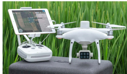
Figure 3. Diagram of DJI Phantom 4 Multispectral. Retrieved from ( https://www.dji.com/cn/p4-multispectral , accessed on 28 August 2024).
