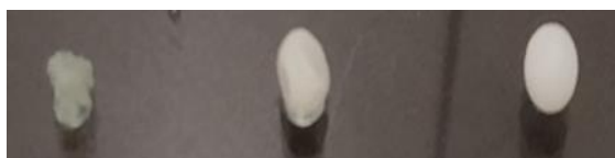
Figure 9 - Different outcomes of hydrogel beads' formation: wrinkled, partially degraded and, spherical, from the left to the right, respectively
