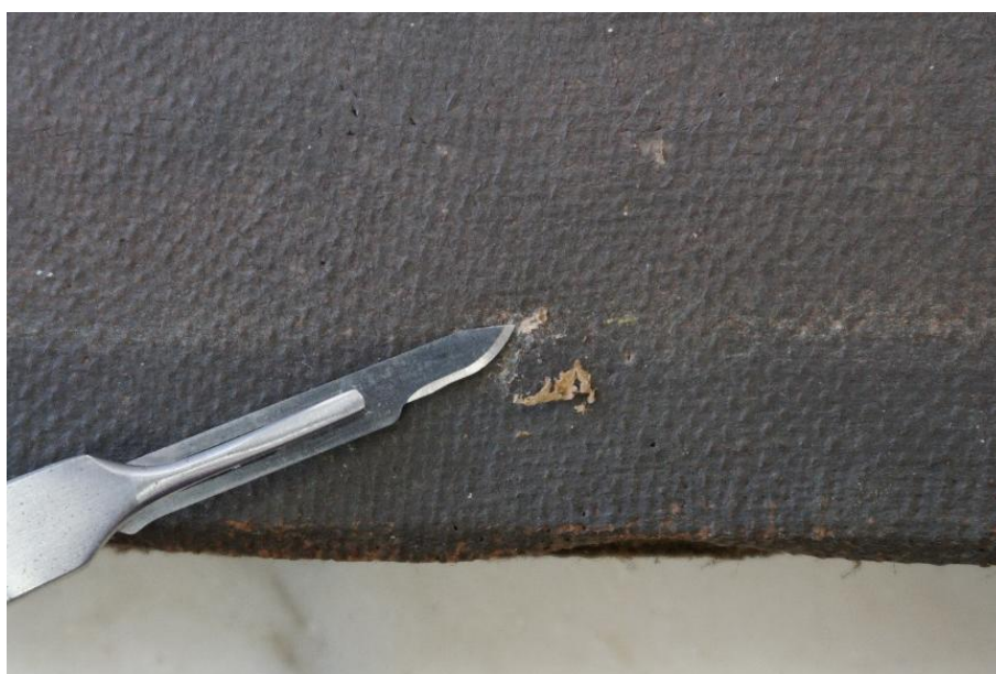
Figure 3.6: Removing deposits with a scalpel.
