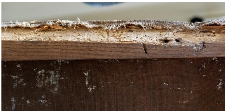
Figure 2.3: Material loss due to xylophagous insects attack.
