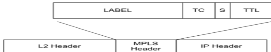
Figure 2.1 IP packet encapsulated by MPLS header.
