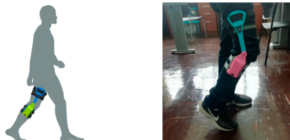
Figure 2.16: 3D printed knee goniometer [58]
