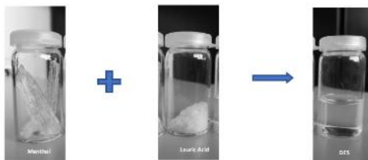
Figure 1.5 — Preparation of NADES from menthol and lauric acid.
