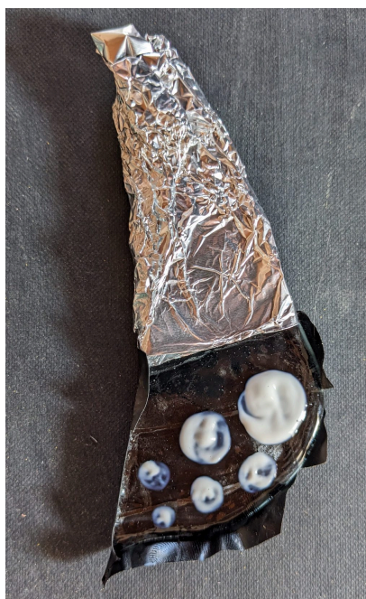
(a) Application of different masking materials to a sample of batch A1 glass.
