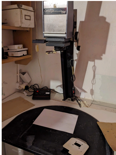
Figure 11: Enlarger for exposing the plates.
