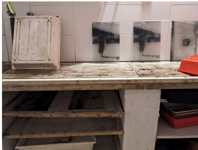
Figure 15: Once the excess water has dripped off the plates are left to dry on the drying rack below the bench.
