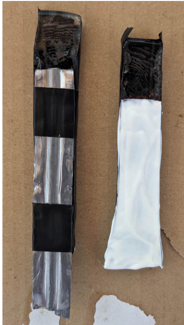
(a) Samples of glass A1 masked with lead came (left) and SPF50 sun cream (right).
