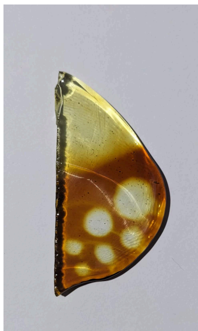
(b) The same sample after undergoing 5 days of exposure in sunlight and development heat treatment for 1 hour at 600°C.
