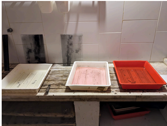
Figure 13: From right to left: developer, stop bath and fixer trays.
