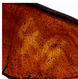
Figure 35: The A4-Br sample with '4H' visible where the permanent marker unintentionally acted as an exposure mask.
