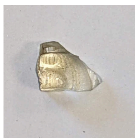
Figure 24: The A3 sample exposed to 330nm radiation, after undergoing the first development heat treatment (500°C).
