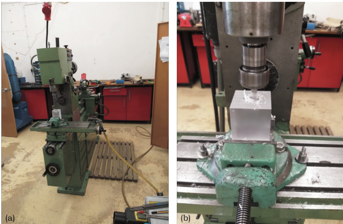
Figure 3.5: Production of the chamber and lid of the ES setup: (a) Milling machine and mechanical lathe; (b) Machining of a PMMA block.
