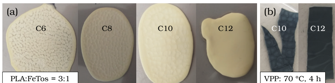
Figure 4.18: Films produced from PLA and PLA/FeTos solutions with a ratio of PLA to FeTos of 3:1. (a) PLA/FeTos films; (b) VPP results from 4 h of exposure to EDOT vapors, at 70 °C.
