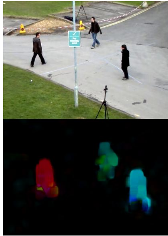
Figure 2.5: An example of Farneback Optical Flow, taken from [29]
