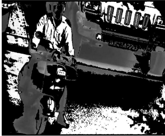
Figure 3.2: Subtraction of the vehicle image from the mean background image, taken from [41]
