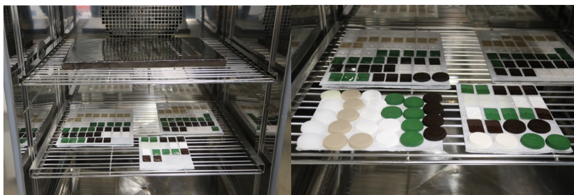
Figure 15. Model painting, rectangular samples and circular samples inside the environmental chamber. For trials 2-5, the samples were placed on a glass plate partially covered with a Reemay® 2004 acid-free polyester tissue 17 . The Reemay® was not completely attached to the glass, allowing for air to circulate under the samples.
