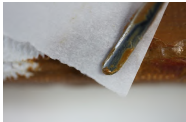
Figure VIII. 37. Process of mattifying the NOVA-PWR infill with a sheet of baking paper and a spatula
