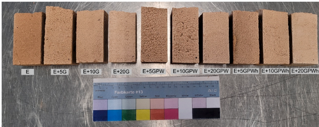
Fig. 5. Colour of mortars with 0 %, 5 %, 10 % and 20 % vol. addition of G, GPW and GPWh. (For interpretation of the references to colour in this figure legend, the reader is referred to the Web version of this article.)
