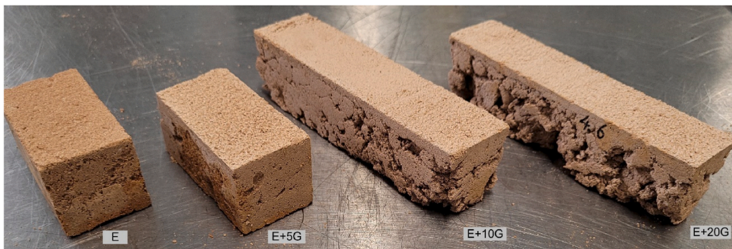
Fig. 6. Specimens of the reference earth mortar (E) and earth mortars with 5 %, 10 % and 20 % vol. of raw hemihydrate (G), showing the lack of compactness of the ones with higher content.
