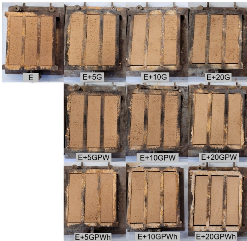
Fig. 7. Observation of the specimens' shrinkage in the moulds, showing the shrinkage increase with gypsum-based binder contents.
