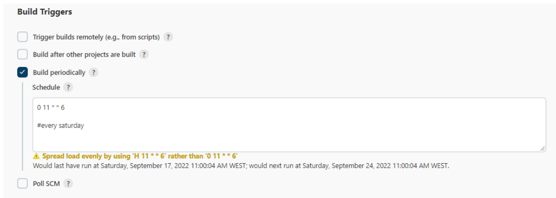
Figure 4.16: Jenkins Scheduling Configuration
