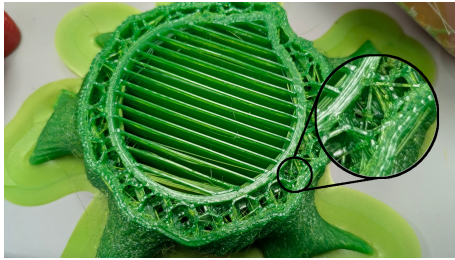
(a) Over Extrusion anomaly.
