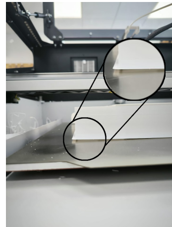
(d) Warping anomaly, the base of the print part is detached from the print bed.
