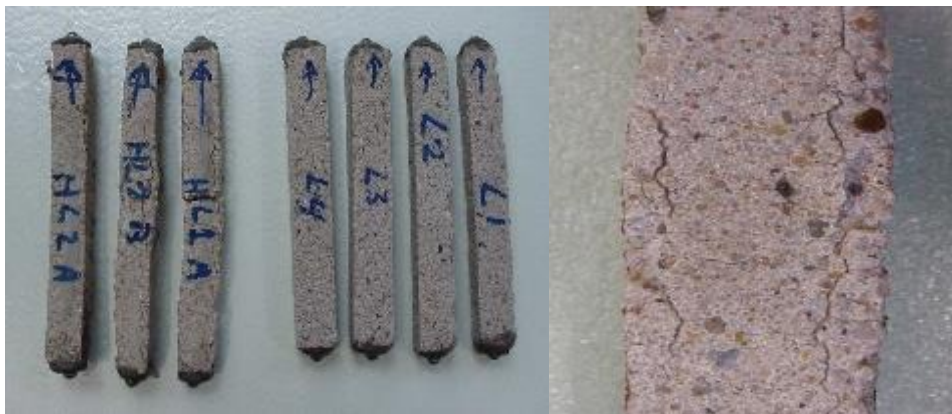
Figure 20. Mortar prisms after 15 weeks in sulfate solution. Natural Hydraulic Lime based (NHL) specimens with clear expansion and deformation and Hydrated lime based (CL) without any expansion, from [72]. HL = natural hydraulic lime (St Astier), to the left; L = hydrated lime based, to the right; picture on the right = detail HL.
