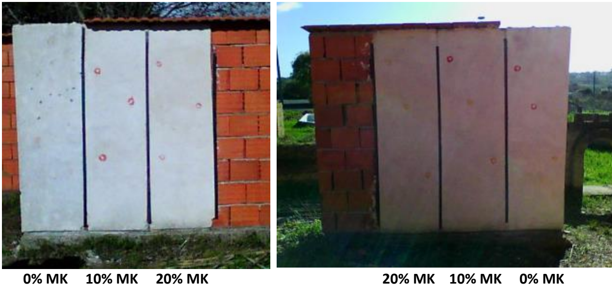
Figure 4. Experimental pure air lime renders and air lime-metakaolin (MK) renders (with the percentage of MK replacing lime) after 7 years of natural exposure (a) South and (b) North, in a semi-urban environment 3 km far from the Atlantic Ocean.
