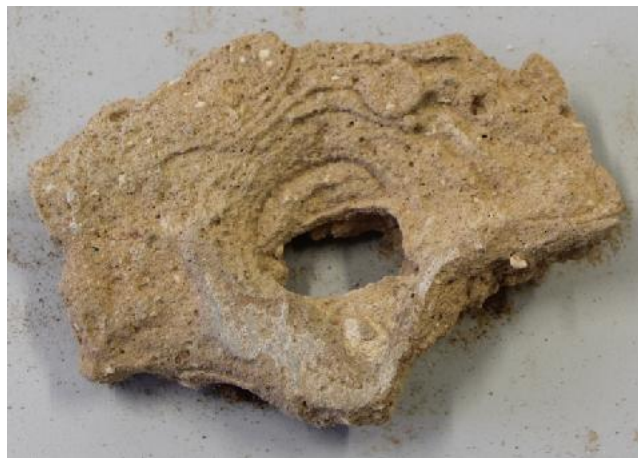
Figure 28. Deep circular erosion on a render sample of Valfiores Palace.
