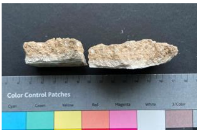
Figure 25. Samples of the old lime render in two coats.
