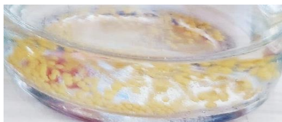
Figure 6.9: No color change that would indicate glutaraldehyde polymerization – Immobilization complex HM 2 after 72 hours of saccharification at 50°C.
