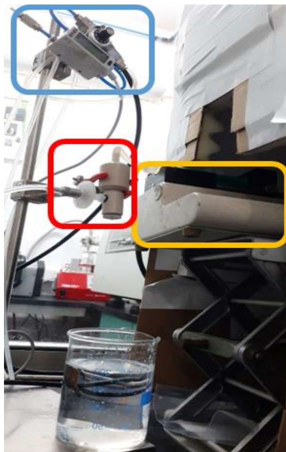
Figure 2.3: Setup of coaxial airflow dripping bead generator system. This system consists in a coaxial airflow dripping bead generator (in red), controlled by an air pump (in blue), and fed by a syringe pump (in yellow). The final part of the setup consists in a precipitation cup filled with NaOH solution, in which the droplets are formed.
