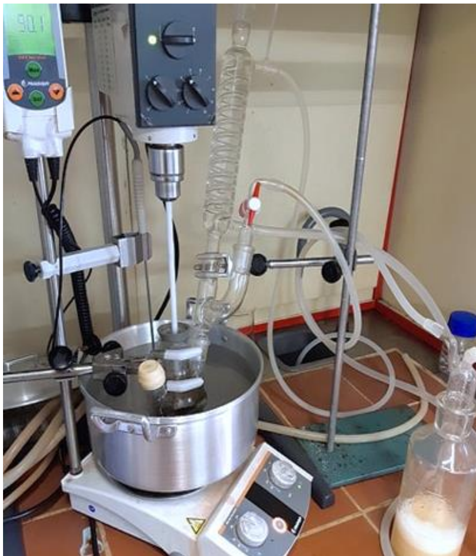
Figure 2.2: Setup for ATPES' coating of SPIONs. The precursors are placed in a three-neck round-bottom flask, with mechanical stirring on the middle neck. An adaptor is placed in one of the lateral necks, and both a condenser and the N 2 hose for mimicking an anaerobic atmosphere are assembled. The other neck is covered by a cap to maintain the N 2 atmosphere. The flask is then set on an oil bath that is maintained at 90 \pm 0.5 °C.
