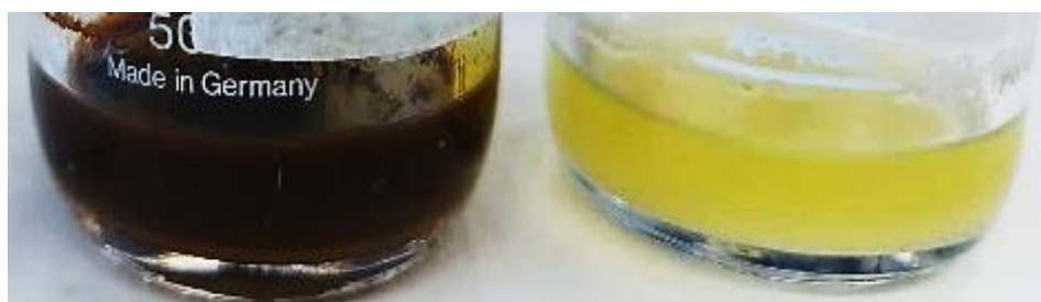
Figure 6.6: CAS 3 (left) and CAS 2 (right) after 1 saccharification cycle of 72 hours at 50 °C. The integrity of CAS 3 was maintained, presenting the dark color that is characteristic of the SPIONs' matrix. Contrarily, CAS 2 presents a bright yellow color and, thus, denounces the loss of integrity of the Fe 3 O 4 that constituted the SPIONs that constitute the core of the matrix.
