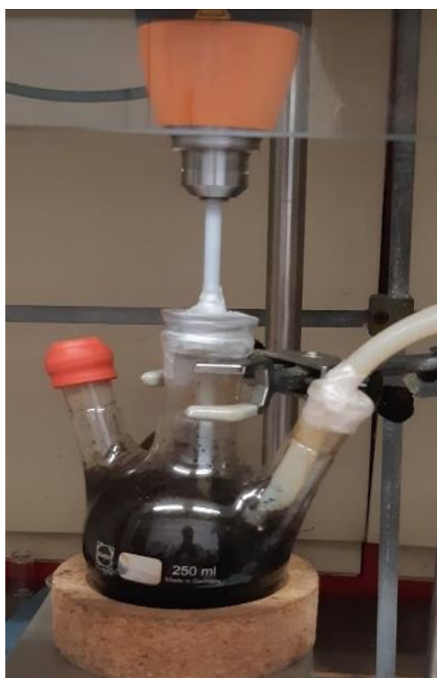
Figure 2.1: Setup for SPIONs synthesis. The precursors are placed in a three-neck round-bottom flask, with mechanical stirring on the middle neck. An anaerobic atmosphere is mimicked by bubbling \text{N}_2 onto the solution by a tube through one of the lateral necks, while the other neck is covered by a cap to maintain the \text{N}_2 atmosphere.
