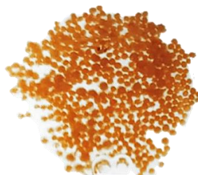
Figure 6.8: Color change caused by glutaraldehyde polymerization – Immobilization complex HM 1 after 72 hours of saccharification at 50 °C.
