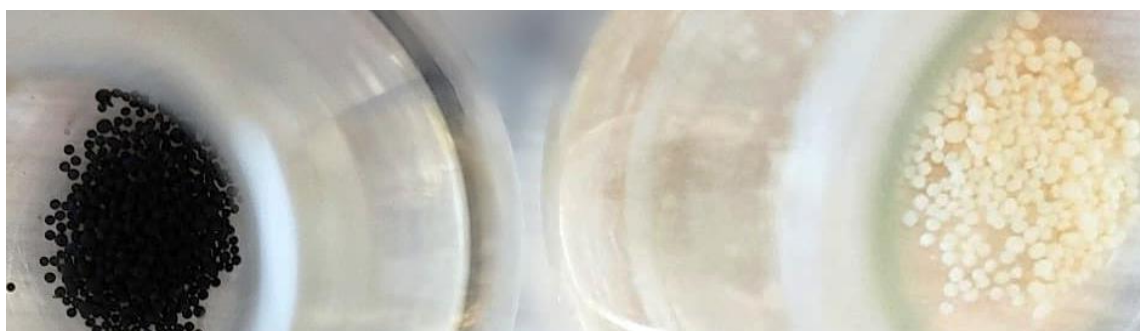
Figure 6.10: CMPs with magnetic cores (left) and the standard non-magnetic CMPs (right). Both batches were produced on the same day and following the same parameters. Due to the increased viscosity that resulted from the addition of SPIONs to the polymer mix, the size of the magnetic CMPs is, on average, visibly smaller.
