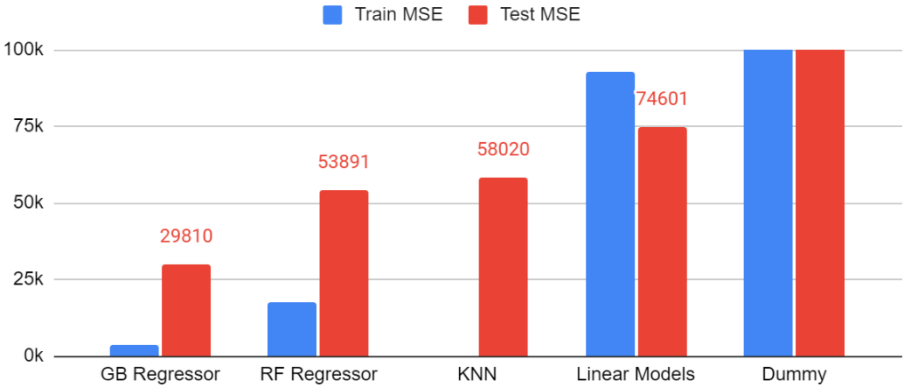
Figure 7 - Model Scores (Causality Framework). For each model, both train MSE (mean squared error) and test MSE are shown. The red label shows the specific value of the test MSE. Models are ordered from best to worst (from smallest to largest error). The Ensemble Tree Models (Gradient Boosting Regressor and Random Forest Regressor) achieved the best score, with a significant difference between the two. The K-nearest neighbors model achieved a score very similar to the RF Regressor. The best linear model performed worse than the other three models and better than the Dummy Model, with a baseline error of over 100'000.
