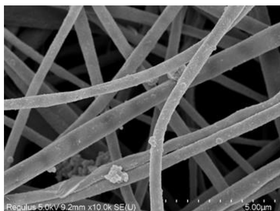
Figure 22: SEM image of PPY/CA fibers after drug release and respective mean fiber diameters.
