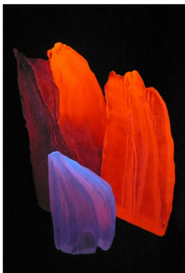
Figure 1.5: Glass sculptures with europium and cerium under UV-light lamp at \lambda = 366 nm [19]
