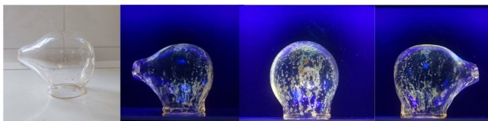
Figure 4.2: Soda-lime glass luminescence piece by Wai in Chan. On the left, the piece is shown under natural sunlight and, on the right, the piece is shown under UV-light lamp at \lambda = 366 nm.
