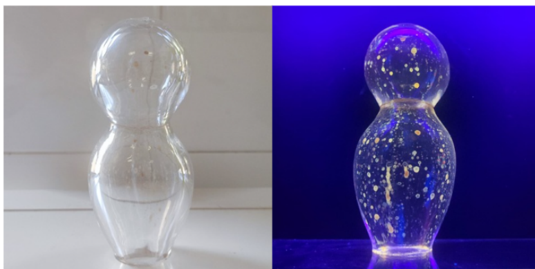
Figure 4.3: Soda-lime glass luminescence piece by Mayank Sahni. On the left, the piece is shown under natural sunlight and, on the right, the piece is shown under UV-light lamp at \lambda = 366 nm.
