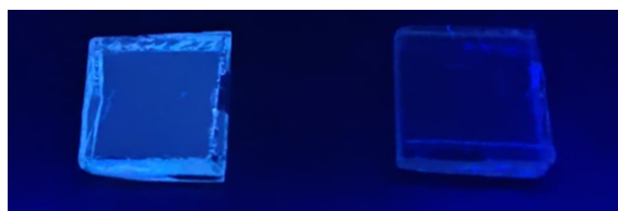
Figure 3.2: Soda-lime glass sample under UV light at a wavelength of 254 nm with tin (left) and without tin (right).
