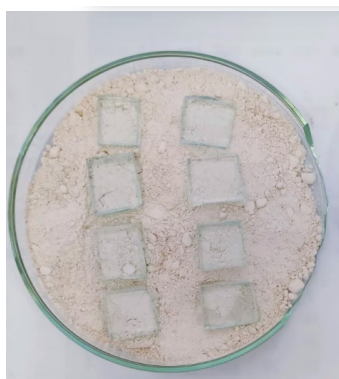
Figure 2.13: Soda lime glass samples on a petri dish a layer of kaolin below. Samples under natural sunlight and before firing
