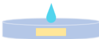
Figure 2.7: Representative Figure of drop casting deposition on glass, in a petri dish. The blue area represents the petri dish, the yellow square represents the glass and the drop illustrates the solution being deposited.
