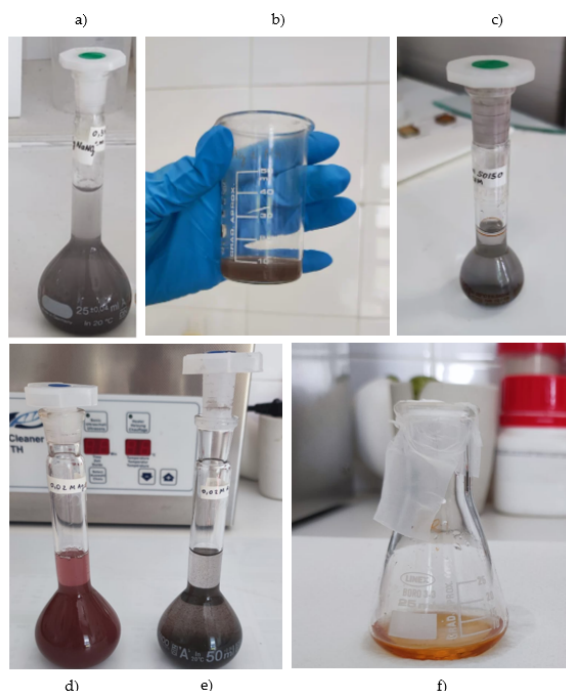
Figure 2.8: Solution tests \text{AgNO}_3 and \text{NaNO}_3 in a) distilled water; b) ethanol; c) 25 mL water MilliQ/25 mL glycerol, f) triethylene glycol monomethyl ether, e) polyethylene glycol 400; \text{Ag}_2\text{SO}_4 and \text{Na}_2\text{SO}_4 in d) decoflux .
