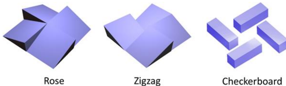
Figure 25: Depiction of different arrangements of diffractive elements (photonic domains) in square lattice structures. The rose (left) and zigzag (center) structures are based on the same diffractive element, i.e. a mono-pitched roof, which is rotated 90 degrees four times. The checkerboard structure (right) results from the simplification of the mono-pitched roof as a non-slanted grating line. Since all photonic domains contain one element, the computational unit cell encloses four.
