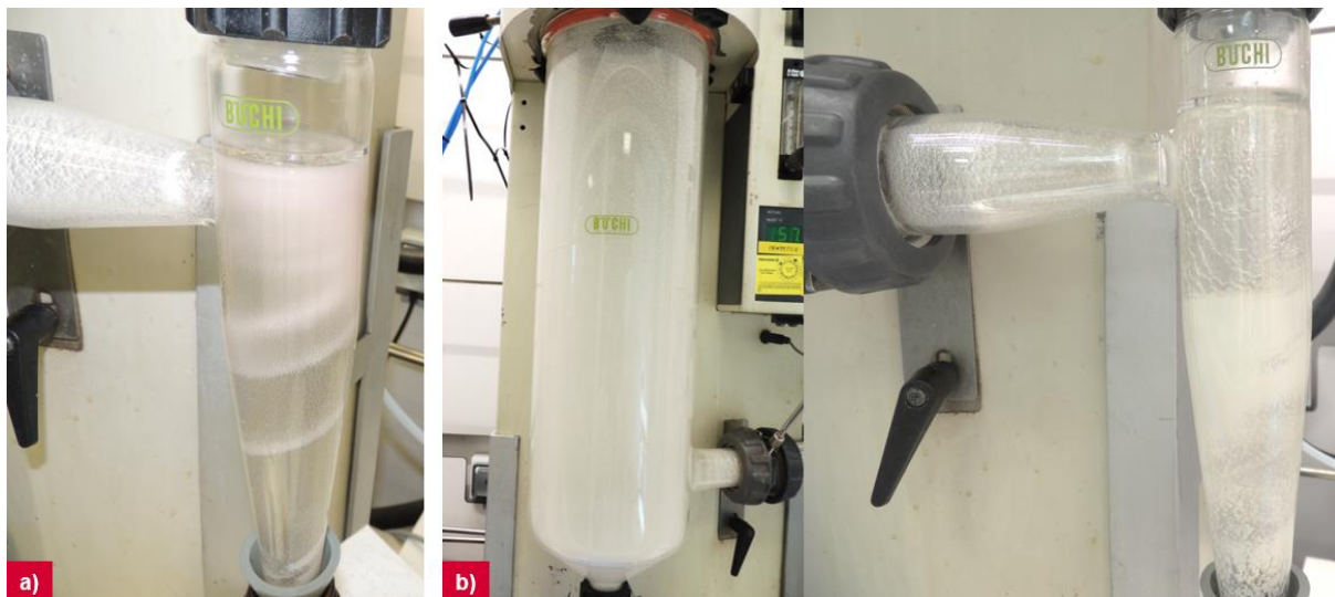
Figure 4.20 – Product accumulation during spray drying. a) first cyclone during ITZ HSM suspension isolation; b) drying chamber and cyclone during ITZ HPH suspension isolation.
