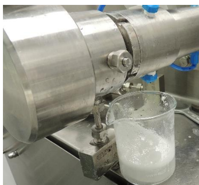
Figure 4.13 – Product losses inside the intensifier pump.
