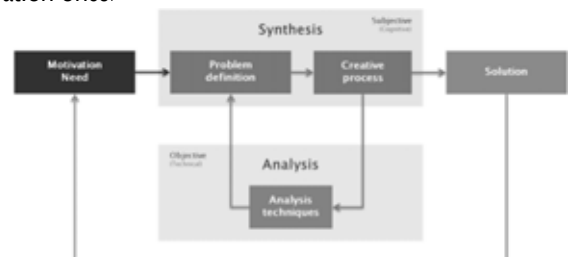
Figure 1 The design process as a feedback system, based on Suh [Suh, 1990].
