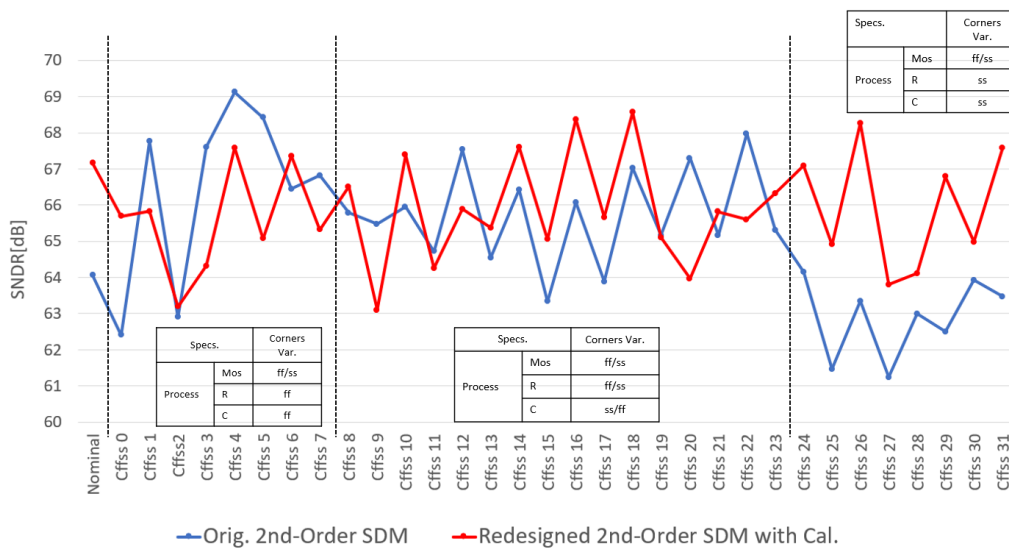
Figure 5.16: SNDR results of the 2 nd - order \Sigma\Delta M, with and without calibration, for the PVT variations, simulated without transient noise.
