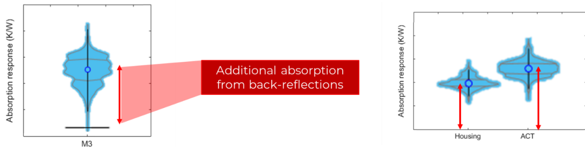
Figure 4.3: Explanation of the back-reflections impact evidence
