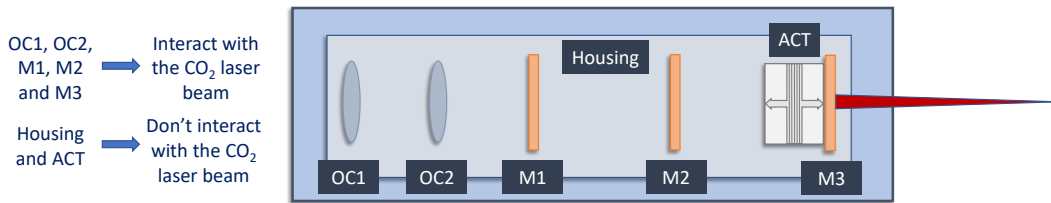
Figure 2.10: Schematic of the order of the structures inside the FO (Not a real representation of their position)
